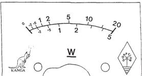
WATTMETER SCALES (5w & 20w FSD) Stick-on Scales 2 supplied with kit These are for use with the stated values of R2 and R3 in the article. Alternative higher (up to about 200w) or lower full scale deflections can be had by changing R2 and R3.
